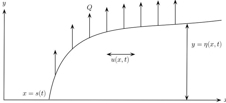
FIG. 1.1. Definition diagram for the slow spreading of a viscous film over a plate with evaporation.
